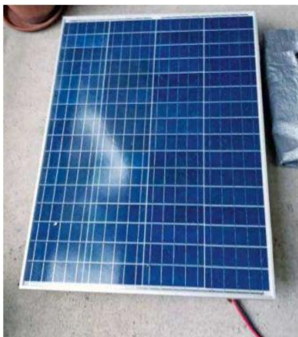
The 12 V 100 W solar panel.
