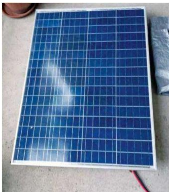
The 12 V 100 W solar panel.
