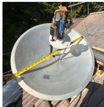
Scott Tilley's, VE7TIL, dish antenna for receiving NASA STEREO-A spacecraft. [Photo courtesy of Scott Tilley]
