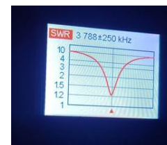
The screen of an antenna analyzer after getting an 80-meter antenna adjusted properly. [Todd Emmert, W9TWE, photo.]
