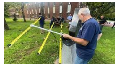
The teachers made tape measure Yagi antennas for the experiment. [Sierra Harrop, W5DX, photo]
