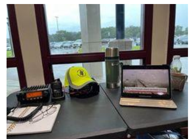
An ARES activation setup at Palm Harbor University High School, one of some 25 shelters in Pinellas County, Florida, providing communications in case of infrastructure failure. Radios communicate directly to the Pinellas County Emergency Operations Center. [ARRL member Stephen Foy, N4FOY, photo]
