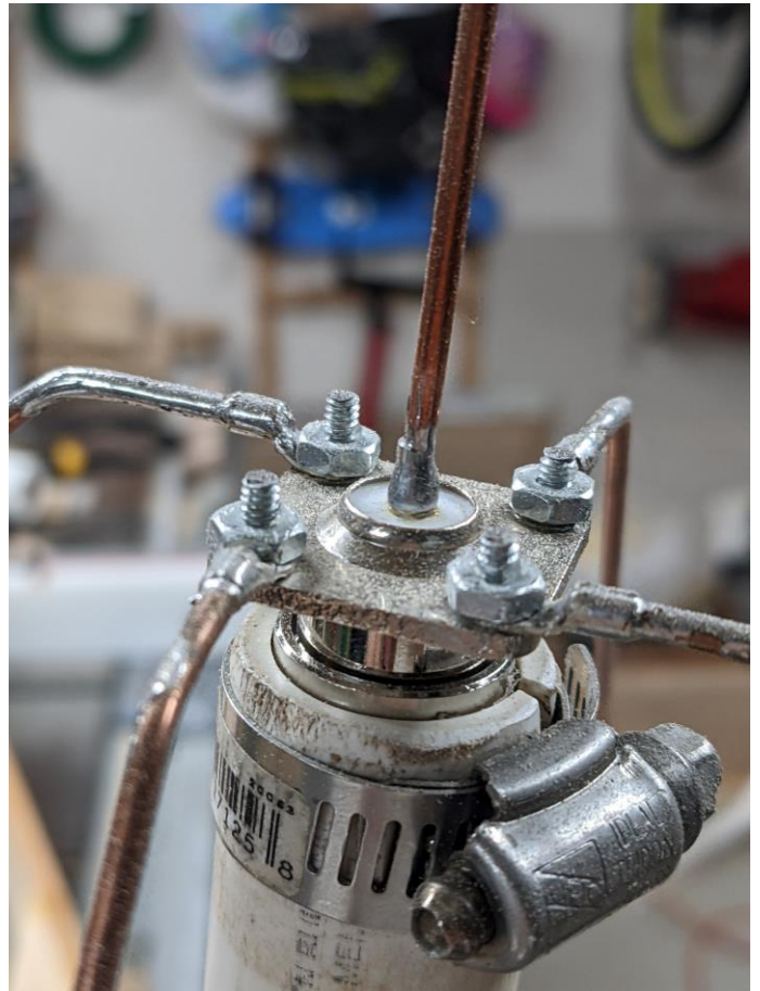
Connections of ring connectors and nuts and bolts. Note: please forgive/ignore the atrocious soldering (I recruited the family to help build this antenna and learn more about radio) and the layer of sawdust on the connector.
