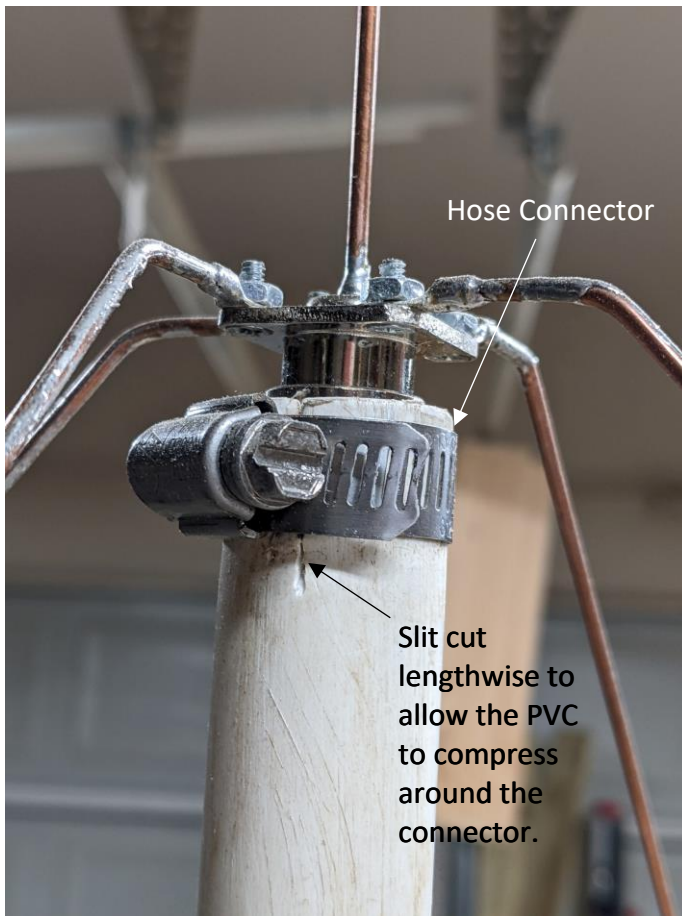
Mast and antenna assembly using hose clamp.
