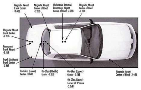
ered when determining the location and type of the antenna. Ground plane requirements vary given the type of mobile antenna and the frequency of operation. A typical 5/8 wave antenna at 150 MHz requires a ground plane of at least 42" in diameter. At 450 MHz, 15" is required, and 800 MHz, a minimum of 8" is considered sufficient.
