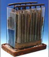
Initial capacity was quite limited since the positive plate had little active material available for reaction. About 1881, Faure and others developed batteries using a paste of lead s for the positive plate active materials. This allowed much quicker formation and better plate efficiency than the solid Planté plate.
