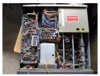
You will find several sub-assemblies. Pick one and start your replacement. I found that by placing your finger on the capacitor you are removing on the top of the board and then placing the finger of your other hand on the bottom of the board helped me find the right pads to de-solder.
