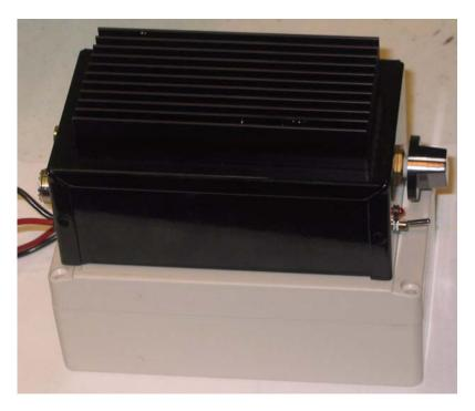
The picture above shows the HF Packer amplifier sitting a top of the new 2-lb battery pack. The high voltage battery pack is 7-times lighter than the average SLA battery pack with equivalent operating time. The higher voltage of this battery makes it possible to offer high/low power modes of operation. This is a safer and superior Lithium Ion battery cell.
