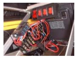
The first photograph shows the basic lay out of the electrical components. The fuse block is from an old car somewhere and contains 4 automotive type fuses. One fuse is 25a for the 100–watt HF rig and the remaining 3 are 15a each for the VHF/UHF rig and accessories. The panel of rocker switches is from a police siren and light control. I chose a terminal strip of sufficient size to allow for distributing the incoming power to the switches, fuses and units.
