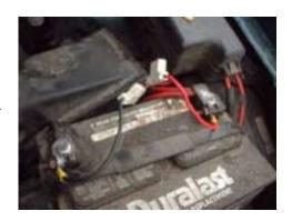
The second photograph shows the connection of the main power cable to the battery with the automotive fuses in both wires. It is always important to fuse both sides of the power cable to your rigs.
