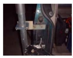
The object was to mount this antenna with out making any visible holes in the body of the van. I think we found a unique method of mounting that many can use. In this photograph, you can see the bolts used to hold the mounts. They are located behind the taillight. Only minor filling of the plastic was required to allow the cables and mounts to use this location.
