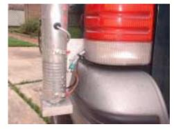
When it comes time to trade in the old 'Mom-mobile', chances are it will never be noticed. The next photograph shows the cables routed through the small opening made with a file. When the antenna mounts are removed, the opening can be filled with black silicon plastic and will be nearly unnoticeable.
