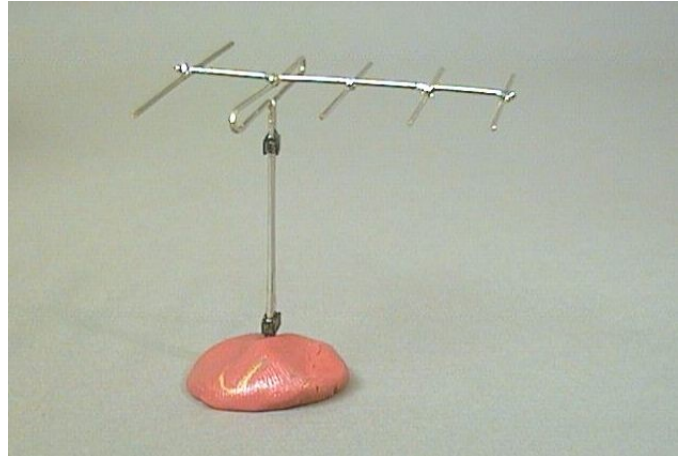
A five element Yagi antenna for 3GHz
